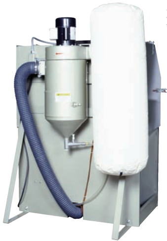
INEX 3048R with 300cfm double-walled dust bag
